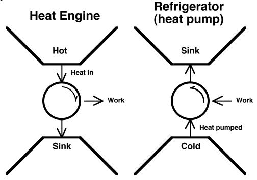
The heat pump absorbs heat at a low temperature, below ambient, and rejects the heat at a higher temperature into the environment through the absorption of work. Here's the important point: <u>work</u> is required to pump the heat from a low temperature to a higher environmental temperature(Scurlock 26).
