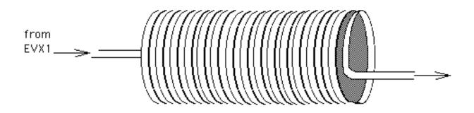
The tube side of the heat exchanger is spiral wound copper tubing and may be more than one layer deep. In HEX I, the tube side is submerged in a liquid nitrogen bath. This is very likely the most efficient style of heat exchanger.
