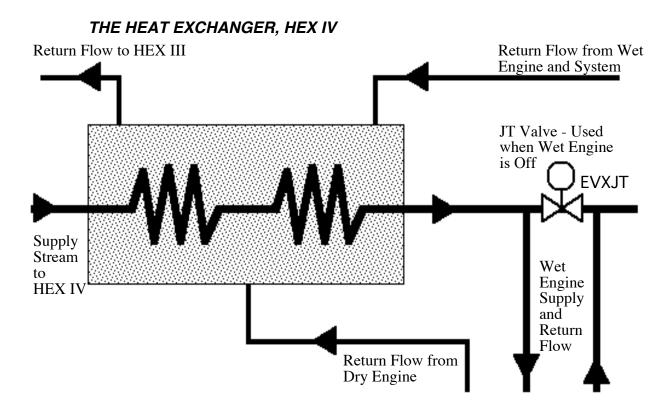
This heat exchanger is also of the tube and shell counter flow design, but its operation is a bit more complicated than the other heat exchangers. Cold gas from the dry engine directly enters the shell side of this exchanger. You may also find liquid helium entering the shell side of this exchanger from the wet engine, the system, or both.
