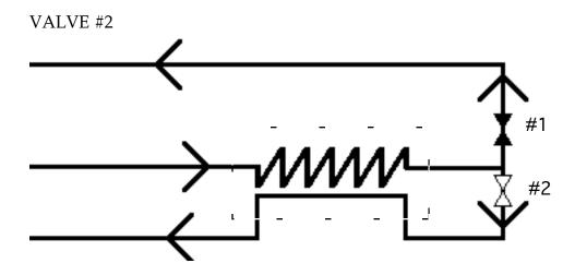
Valve #2: Do you remember this formula, T° in = S° out and T° out = S° in? If you bring a warm gas through the return side, you will simply warm the supply side and the heat exchanger will stay one temperature throughout. In order for a heat exchanger to function properly there must be a differential in temperature — there must be a cold end as well as a warm end.
