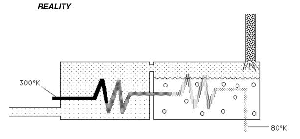
In reality, the liquid nitrogen enters and fills the pot, which covers only the last half of the tube bundle. The cold gas leaving the pot cools the first half of the tube bundle before it exits to atmosphere. This is the way the helium stream initially reaches the 80°K temperature range during cool down.
