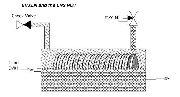
EVXLN: This valve controls the amount of liquid nitrogen flow to HEX I based on the level in the "POT." The  $LN_2$  pot is simply a six-inch pipe mounted horizontally so it can serve as a liquid vessel for the tub side to be immersed in. The other valve is a simple check valve that vents to atmosphere.
