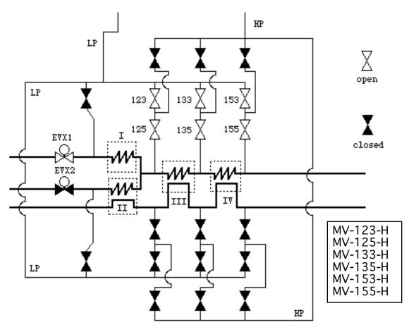
The cool down procedure states that these valves (listed in the bottom corner of the diagram) should be open and possibly throttled.
