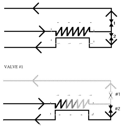
Valve #1: Single pass flow is the proper method of cooling down the heat exchangers. When the tube side is cold, the heat exchanger can be "turned." (This method of single pass flow can also turn a Dewar.) The term "turned" means that the supply flow of gas can give up its heat to the return flow — you don't have a heat exchanger until this is possible.
