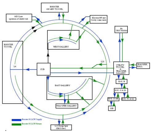
The TeV 95 LCW cools the P2 and P3 line magnets and power supplies.
