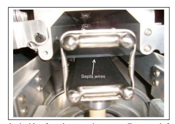
While one can adjust the upstream and downstream ends of septa independently, in practice, the septa should remain relatively level; both the upstream and downstream stepper motors should be adjusted in unison to move the septa parallel to the beam.
