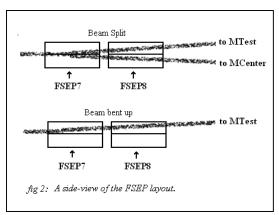
the top of  $fig\ 2$ ). We only run in the configuration where beam is bent up (pictured at the bottom of  $fig\ 2$ ).
