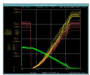
If the apparent transmission as measured by S:F1SEM/I:BEAM21 is less than 75%, there is some anomalous beam loss occurring somewhere upstream (see the <u>Tuning Guide</u>).
